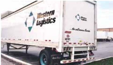
Single-axle pups 12' high 40' long are perfect for site deliveries into tight and/or low-clearance receiving areas
